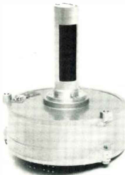
To save weight, an aluminum capstan was used in the drive assembly. A carbon fiber composite surface was added to increase friction and minimize wear.
