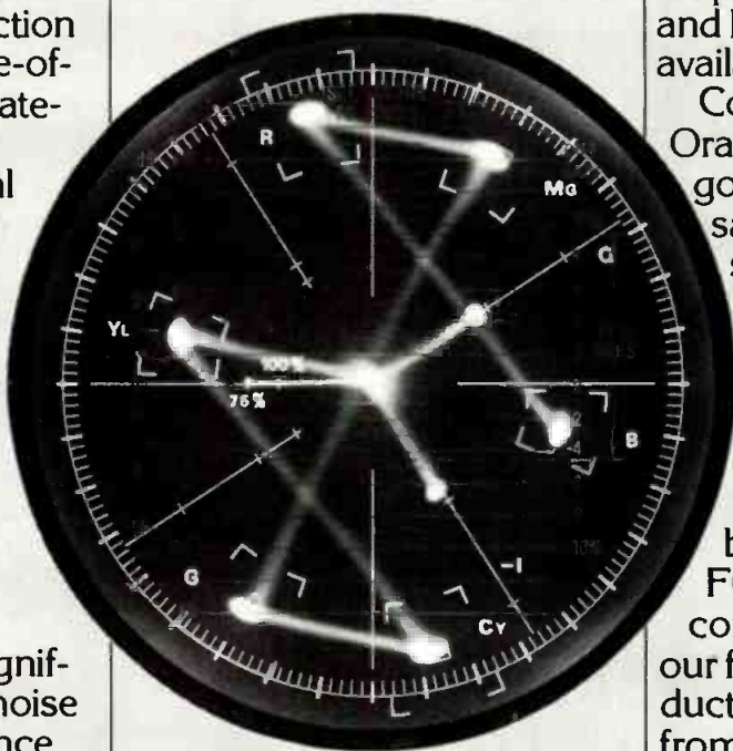
Time base corrected signal input from SONY 820 VTR.
