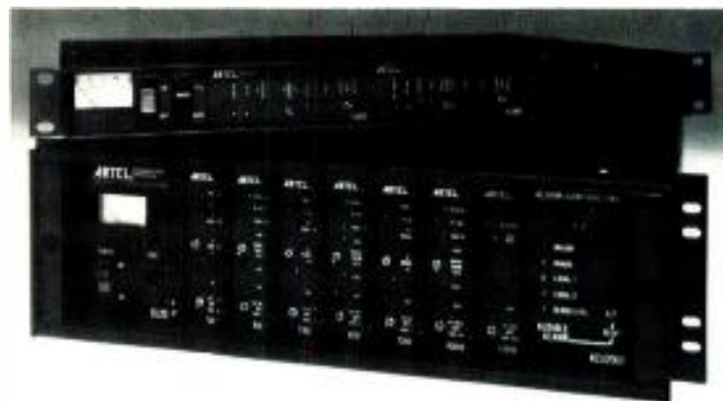
The fiber optic transmission system from Artel intended for production use.
